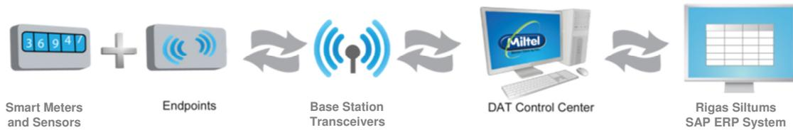
The system incorporates a full two-way communications system supporting all of the customer's data collection requirements as well as a full set of smart grid management tools. The system also supports "over-the-air" updates, whereby Miltel firmware in all of the system components can be modified and upgraded over the network.
